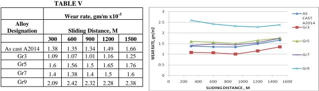
**Fig 3.9:** Wear rate of A2014 and its alloys
